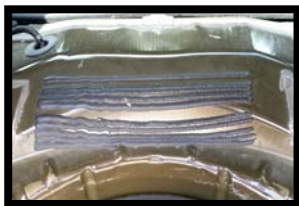
Photos from a 2011 Ford Mustang showing the sound deadener beads placed from the manufacturer in the trunk area.
