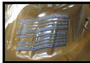
Photos from a 2011 Ford Mustang showing the sound deadener beads placed from the manufacturer in the trunk area.
