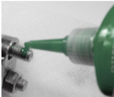
**Note:** Not recommended for pre-assembled threads in a blind hole
