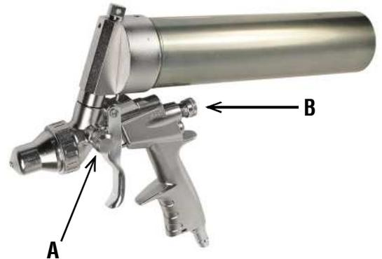
**PLEASE NOTE:** During intermissions of use always keep a cartridge with sealant inside the spray gun, turning the air and product valves to the off position, to keep the product from setting up in the gun. During extended periods of non-use, remove the cartridge and clean the gun immediately. See instructions for maintenance enclosed with the gun.
